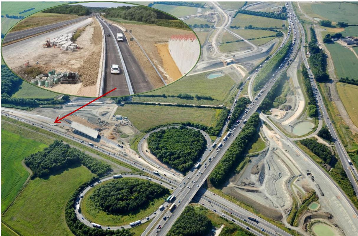
Along the Cambridge Northern Bypass, the lengthy period of night work required for phase 1 of the work will soon come to an end. During this time we have removed the safety barrier from the centre of the road and resurfaced it so we can move traffic over to construct the widened section of this part of the A14. During phase 2 the majority of the work will be carried out during the day.
